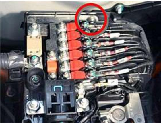
6. Remove the nut that secures the battery fuse box to the battery strap. Tie the battery fuse box aside (torque 6 Nm).
