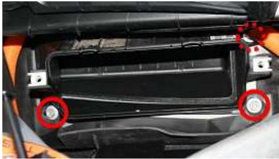
3. Release the lugs (x4) that secure the battery fuse box cover. Remove the cover.
