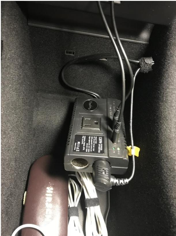
Tuck the wires outside and run them along top left side of the passenger foot well area and stuff excess into the top left corner of the footwell where they were stowed prior with the Blackvue cigarette male and female connectors in prior install. If this is your first install, you can refer to the location where it's easy to tuck and stow excess wires.
