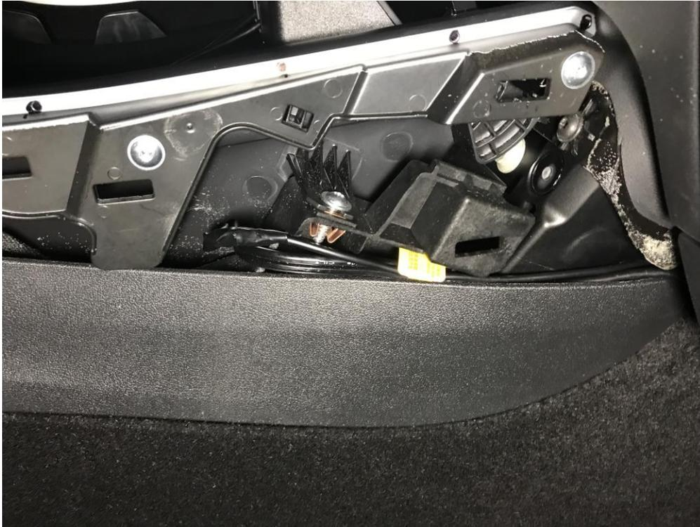
After you're routed and tucked the wires, put the panel back starting from the rear moving forward as you push in the clips. Here's the completed look.
