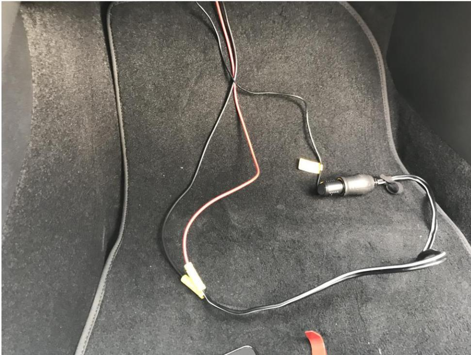
The black and red leads are coming from the Tesla Model 3 12V battery with 15A fuse. The female cigarette receptacle was removed so imagine the red and black leads not terminating at the little yellow re-useable connectors. The Blackvue power cable with cigarette plug was cut off and re-connected inside the console.
