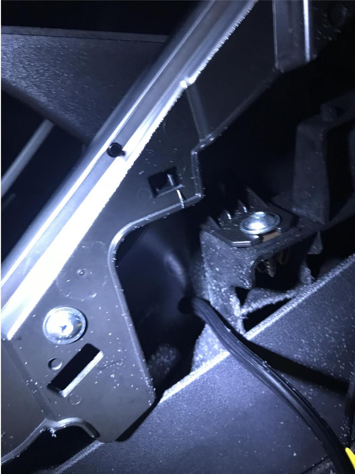
Here's a picture of the cable from the inside of the console. Those two wires shown plugging into the USB ports of the little Tesla's power panel are the two wires provided with the car. You can also see the two USB connectors that come with the car but turn off when the screen goes off. Again the plastic specks were cleaned out afterward.
