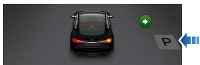
**Note:** The parking icon appears only if the vehicle's position and/or the circumstances of the surrounding area are such that Autopark can determine an appropriate driving path. If Autopark cannot determine an appropriate path (for example, when driving on a narrow street where moving into the parking space causes the front of the vehicle to extend into the adjacent lane), you can either reposition the vehicle, find a different parking space, or park manually.
