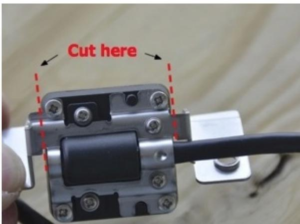
The camera mounts on the center upper front grille just under the nose cone. While the photo shows some of the grille elements cut out, no alterations to the grille are necessary. To mount the camera in this position, the two wings on the metal camera mounting bracket must be first cut off. Using a Dremel tool with a cut off disc or a hack saw, cut the mounting bracket as indicated in the photos below.
