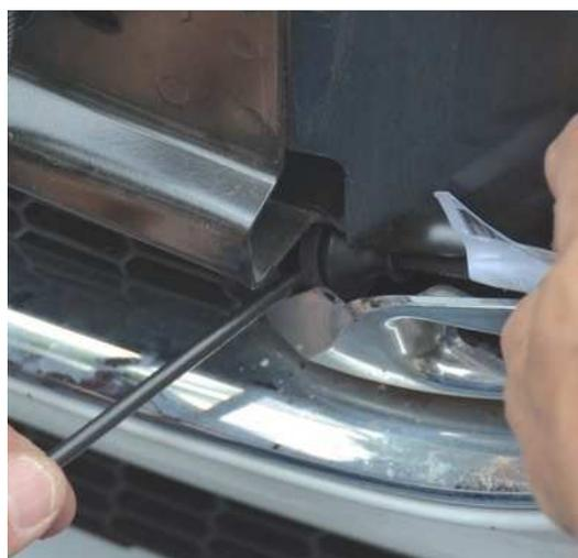
Next carefully thread the other end of cable into the channel slots along the top of the fender to the front of the car in the nose cone area. This will hide the cable and makes for a much easier and neater installation. Next thread the cable through the openings behind/around the right side of the nose cone near the fender channel.
