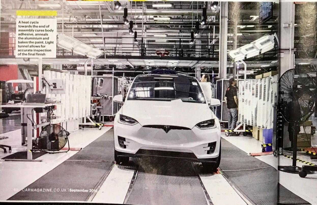
A heat cycle towards the end of assembly cures body adhesive, anneals the aluminium and bakes the paint. Light tunnel allows for accurate inspection of the final finish
