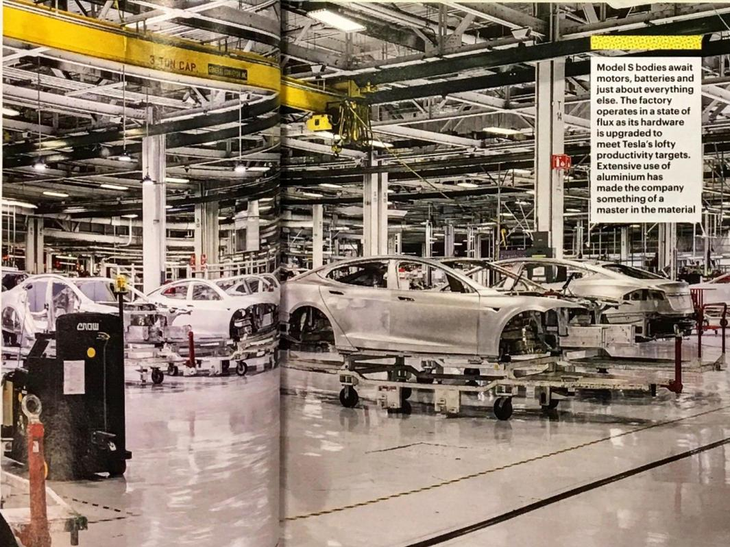
Model S bodies await motors, batteries and just about everything else. The factory operates in a state of flux as its hardware is upgraded to meet Tesla's lofty productivity targets. Extensive use of aluminium has made the company something of a master in the material
