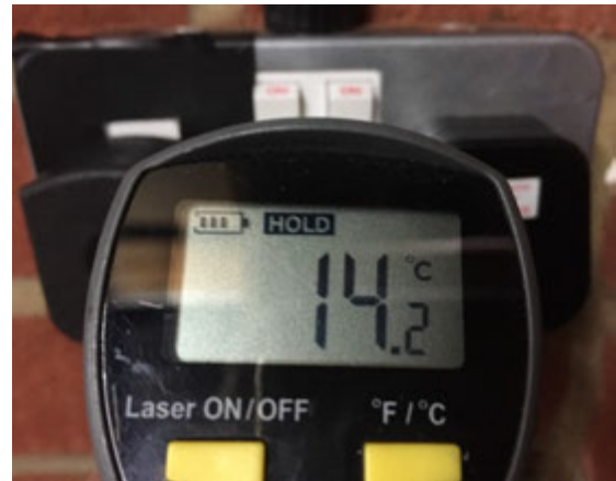
Figure 60 – Temperatures after 30 minutes charging at 13A showing the expected modest increases
