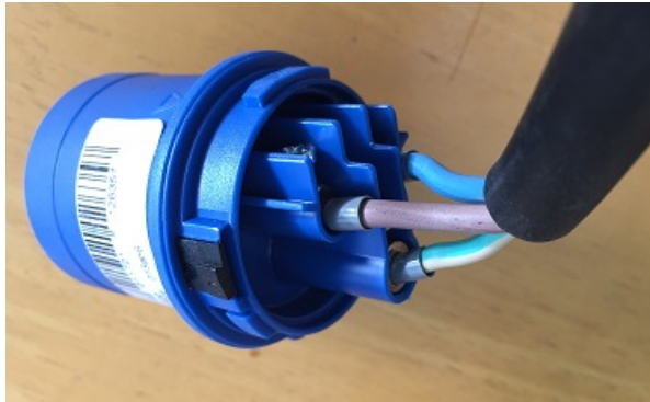
Figure 38 – Wiring of the 16A single phase blue plug
