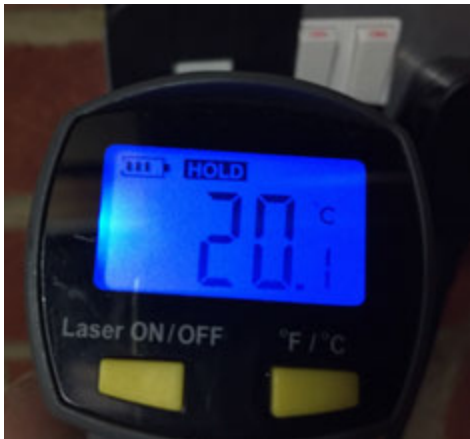
Figure 60 – Temperatures after 30 minutes charging at 13A showing the expected modest increases
