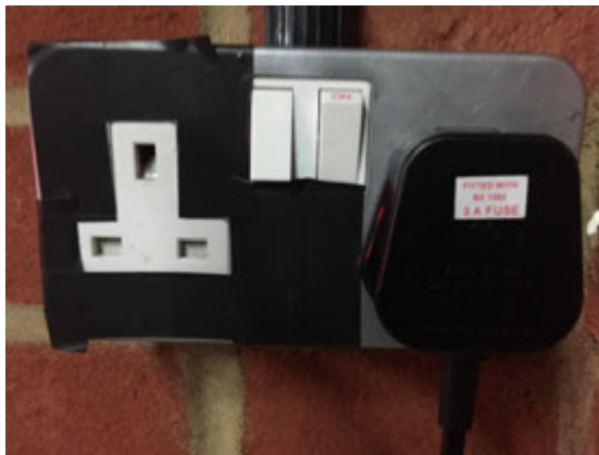
Figure 58 – Insulating tape on the socket face to allow accurate temperature measurement
