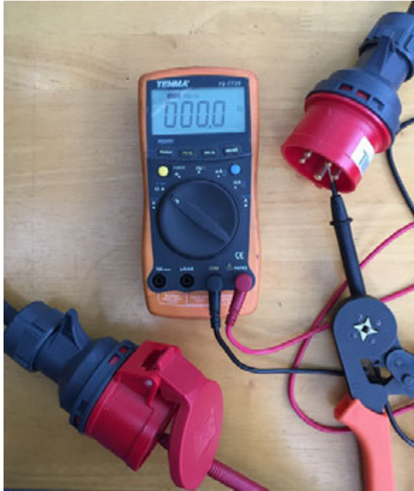
Figure 24 – Measuring electrical resistance
