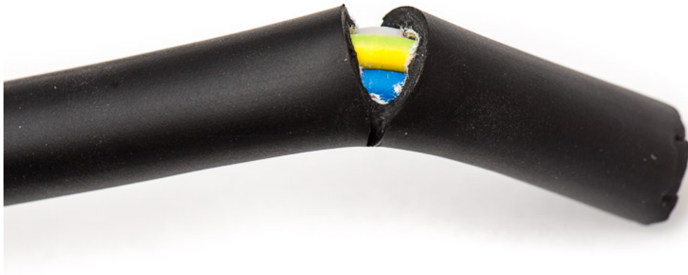
Figure 13 – First cut to remove insulation
