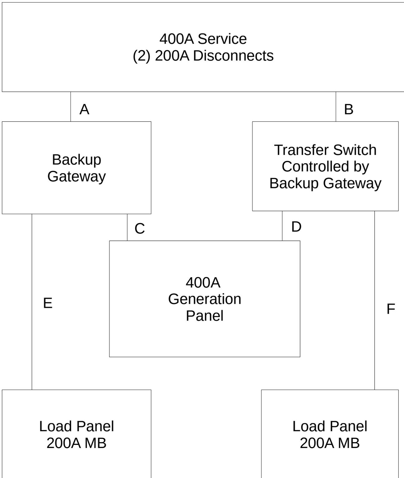
All feeders 200A. Feeder C is monitored by the Gateway CTs to limit export to 200A. The transfer switch connects B to F during normal on grid operation; and D to F when off-grid.
