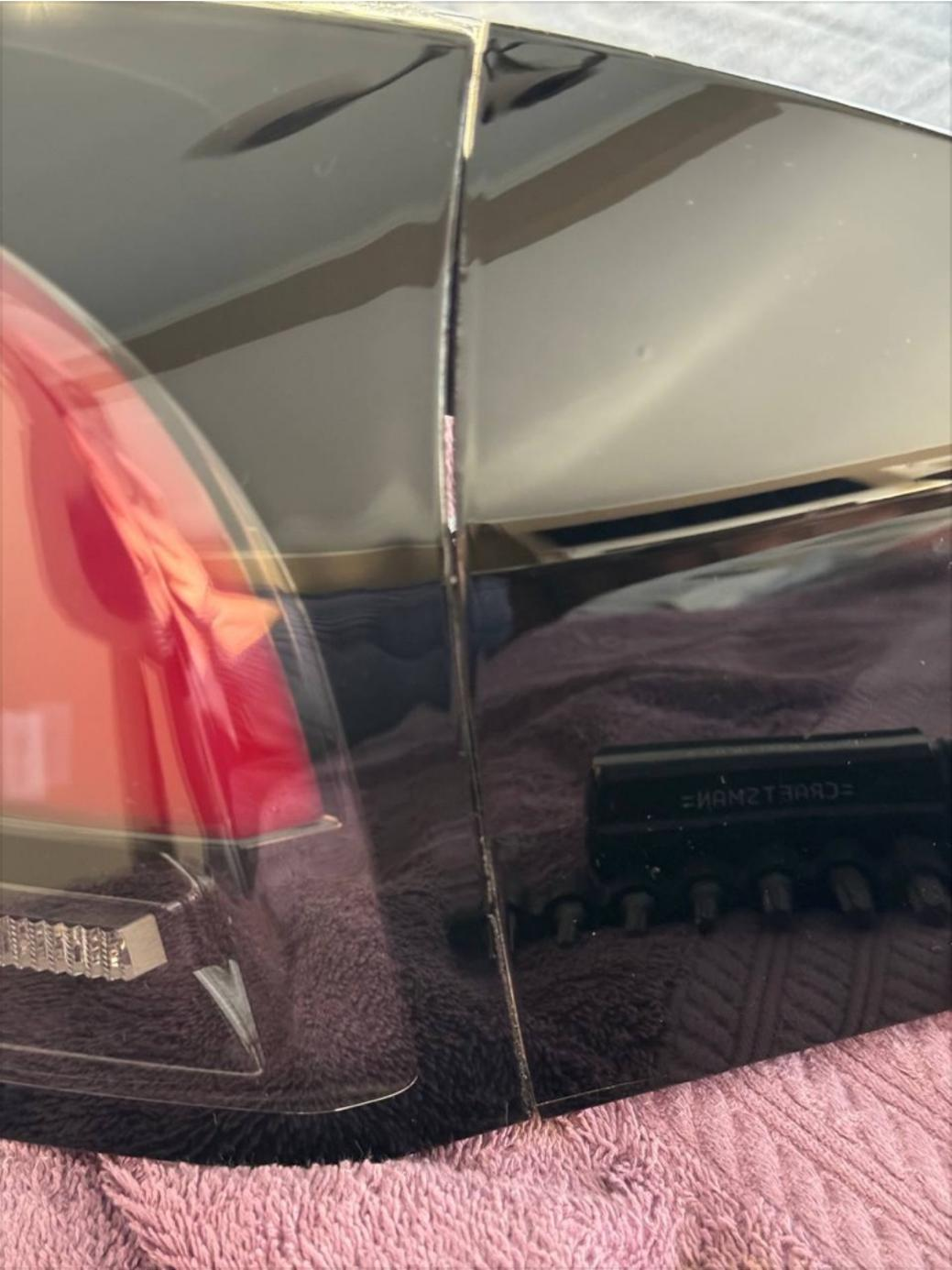
Here you can see how water could get into the light and into the car between the seam. The cut line for the old housing isn't sealed at all.
