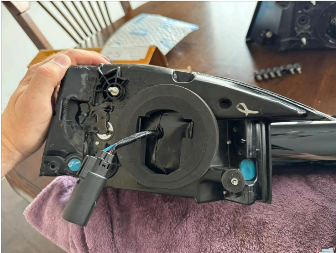
I also transferred the installed rubber boots and spacers onto the EVOffer lights as they were on the existing light. I'm sure someone in the factory was using them to shim the parts into place and make them work with the body.
