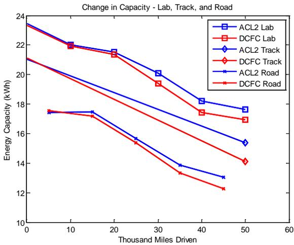
Figure 20. Battery capacity measured or inferred by three methods: lab capacity testing, track constant speed range testing, and on-road data energy usage.
