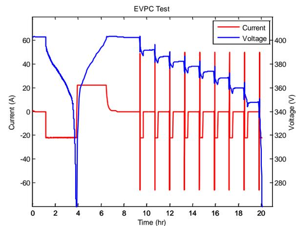
Figure 4. Current and voltage traces for an EVPC test conducted for one of the AC level two control group vehicles are shown
