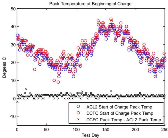
Figure 10. Battery pack temperatures at beginning-of-charge is shown for an alternating test pair of one ACL2 vehicle and one DCFC vehicle over 250 consecutive test days.
