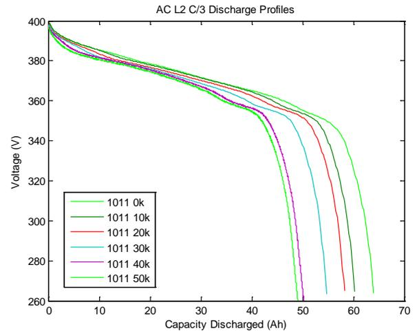
Figure 3. The voltage traces of several constant current discharge tests for one of the AC L2 control group vehicles (VIN ending in 1011) is shown. The area under each curve indicates the energy discharged during the test.
