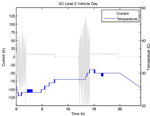
Figure 5. A 24 hour period is shown for an ACL2 vehicle (1011), with the time beginning at the start of the morning drive. Battery current and battery temperature are shown.
