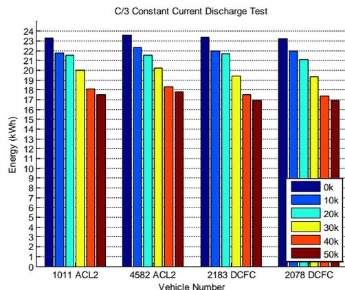
Figure 13. Battery capacity discharged for each pack at 10,000 mile intervals. Each
