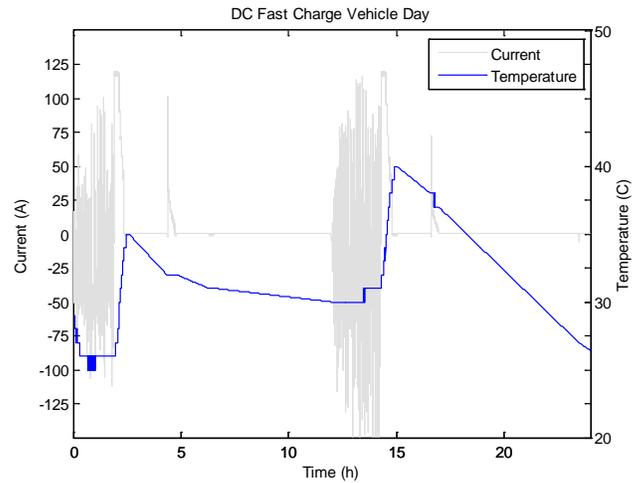
Figure 6. A 24 hour period is shown for a DCFC vehicle (2078), with the time beginning at the start of the morning drive. Battery current and battery temperature are shown.
