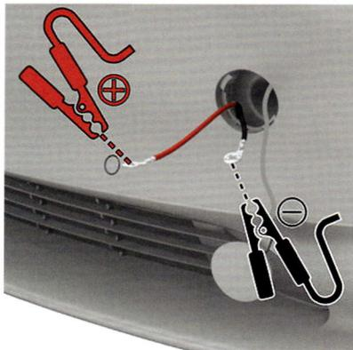
**Note:** Applying external 12V power to these terminals only releases the hood latches. You cannot charge the 12V battery using these terminals.
