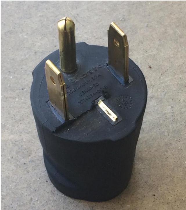
Rather than modifying your Tesla NEMA 14-50 adapter, you could instead modify a 50A NEMA 14-50 extension cord. That would allow you to plug into NEMA 14-60s farther away. However if you do that, you will never be able to use the NEMA 14-50 extension cord as an RV extension cord.
