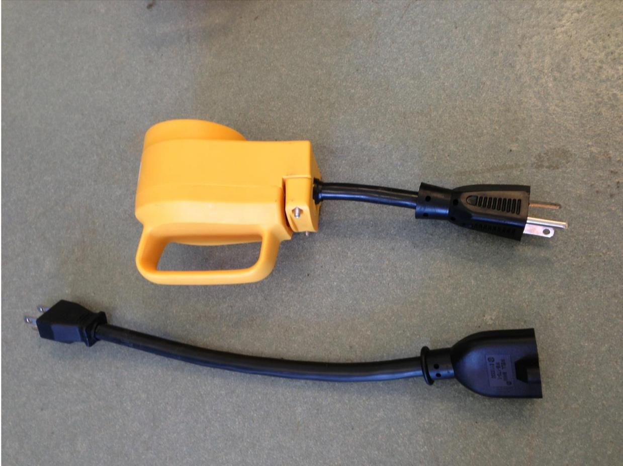
That second pigtail is a NEMA 5-20 to NEMA 5-15 adapter. Sometimes in homes, you have plugs that are connected to 20A breakers, have 20A wiring, but the electrician put in a 15A plug. In theory, you could use that pigtail to draw 16A from such a plug, but now you are pushing it since the wall socket isn't rated for 16A. If you want this last pigtail, you can get it here:
