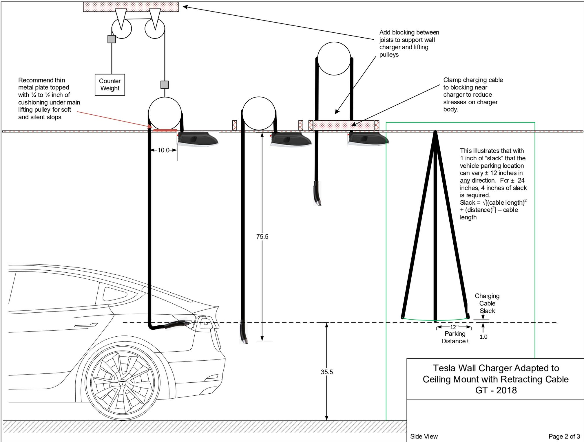
Tesla Wall Charger Adapted to Ceiling Mount with Retracting Cable
