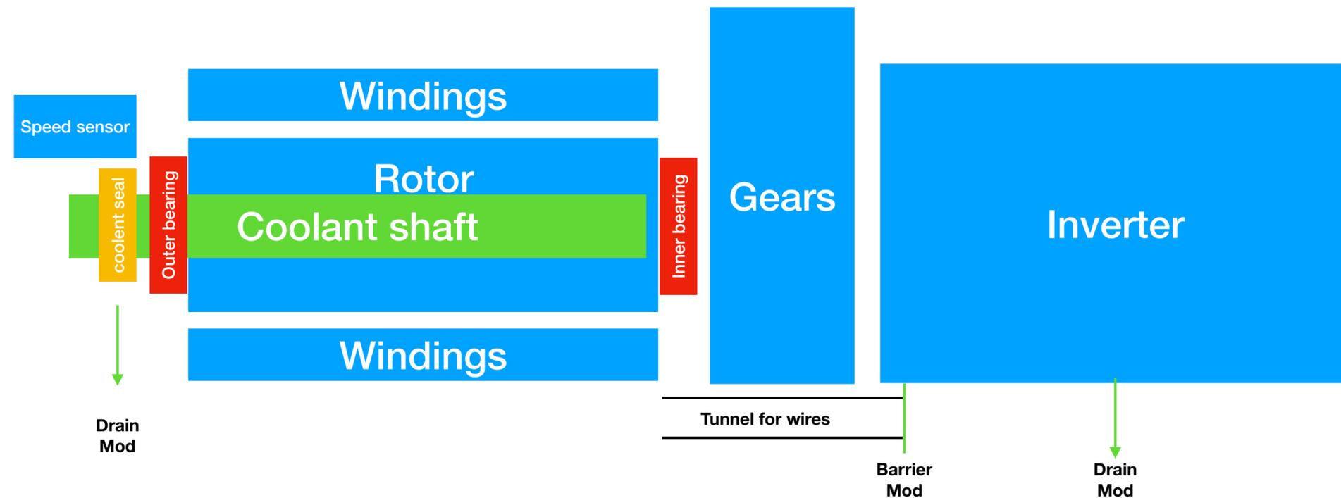
**Coolant goes to the center of the rotor through a shaft to cool it.**
