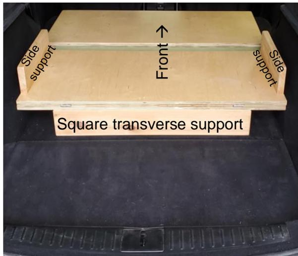
Both sections folded to show three of the four supports. Deep trunk compartment access is preserved. With the front section folded, the front seats can be adjusted over their full range.
