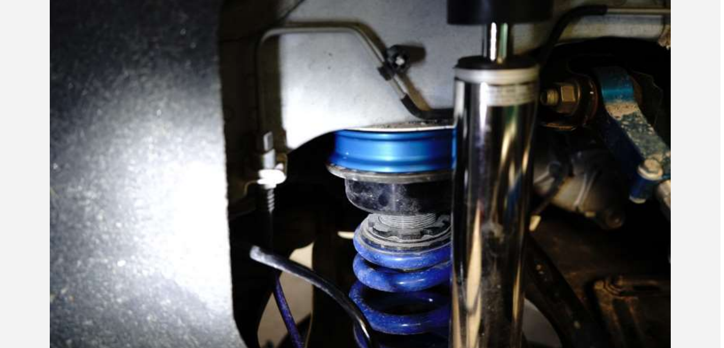
Rear spacer installed in combination with our coilovers. The stack-up order from bottom to top will be: stock rubber isolator, spring, stock rubber isolator, spacer, spacer gasket.
