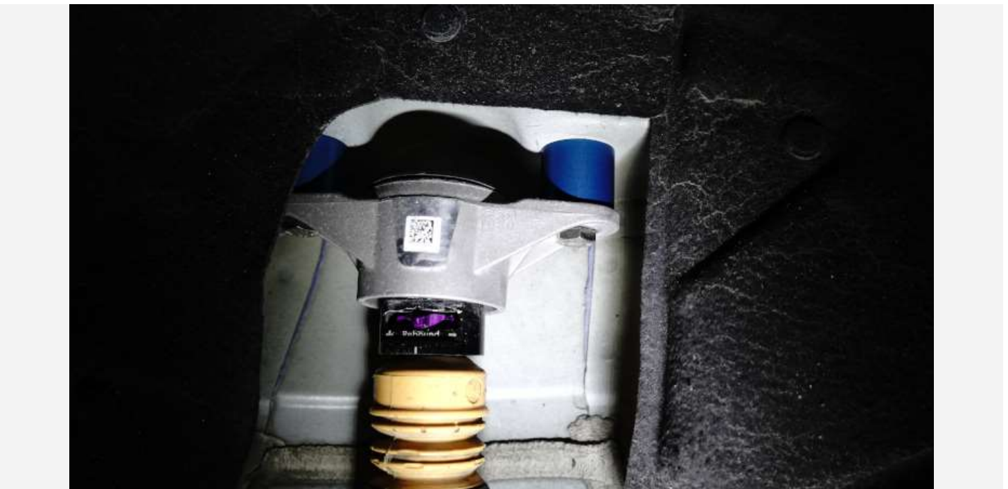
Rear damper installed in car with provided spacers and bolts.
