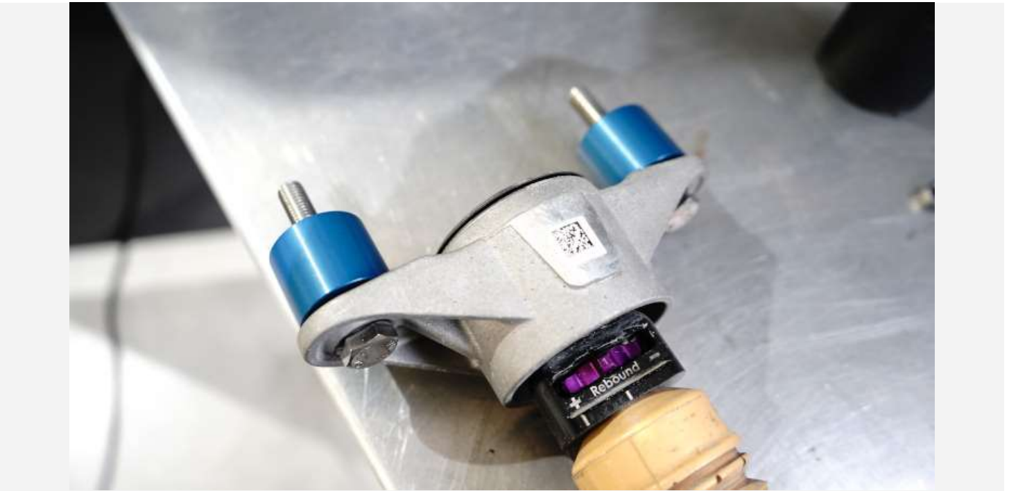
Rear damper spacers installed on top of rear damper mount using longer M10 bolts.
