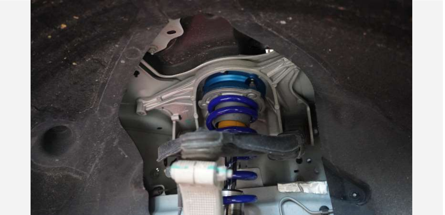
Front damper installed with lift kit spacer. Pretty isn't it?
