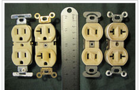
Common 125-volt receptacles in general use throughout North America. All accept a 1-15P plug, and the two on the left accept a 5-15P plug. The NEMA 5-15R device on the far left is most common.
