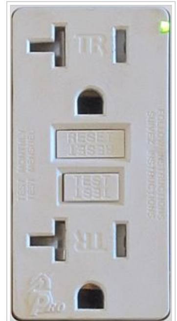
Tamper-resistant GFCI duplex receptacle type 5-20RA, can take 5-15 and 5-20 grounded plugs and 1-15 ungrounded plugs
