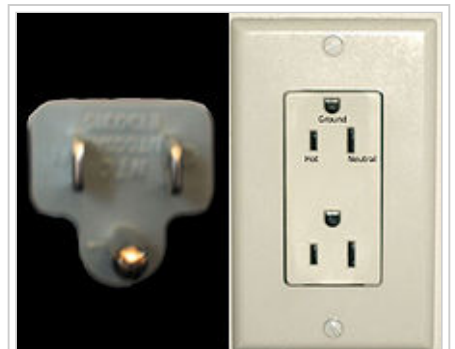
NEMA 5-15P plug and NEMA 5-15R receptacle (different scales, blade spacing is 0.5 inches (12.7 mm) for both.) Each receptacle also accepts an ungrounded plug, whether polarized or unpolarized.
