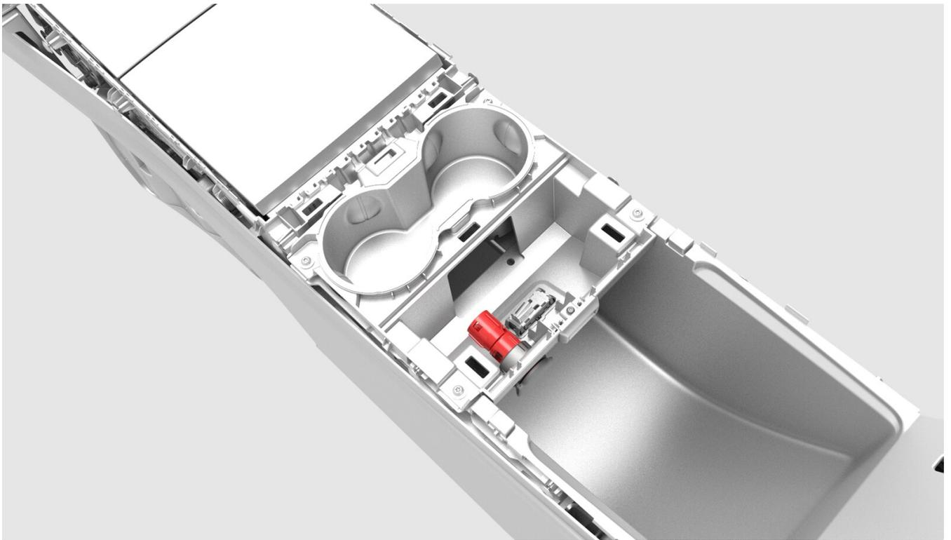
**9.** Release the tabs of the cap and move the power socket and cap together out through the cupholder assembly.
