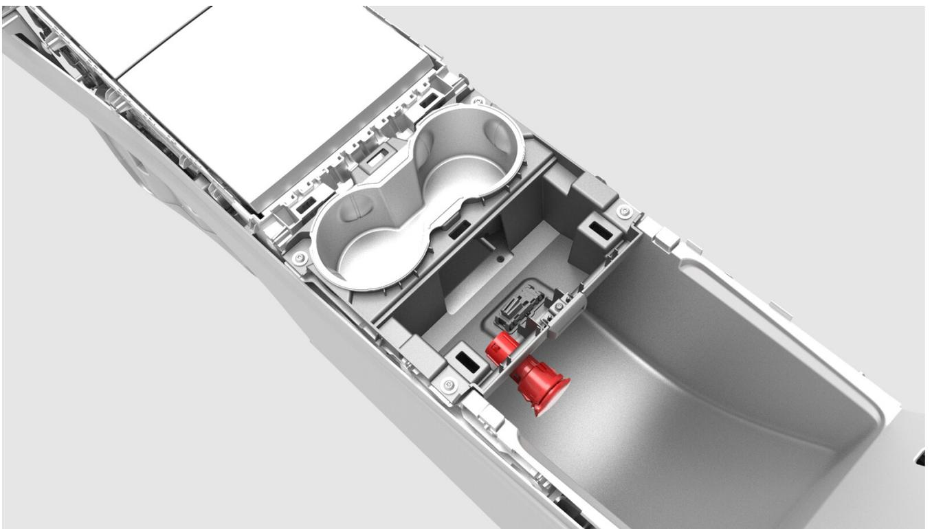
**10.** Separate the power socket from the cap.
