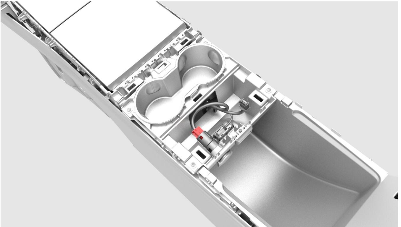
**8.** Release the small tabs on the spring cap and slide the power socket inside the cap, so that the openings in the side of the socket align with the large tabs of the cap.
