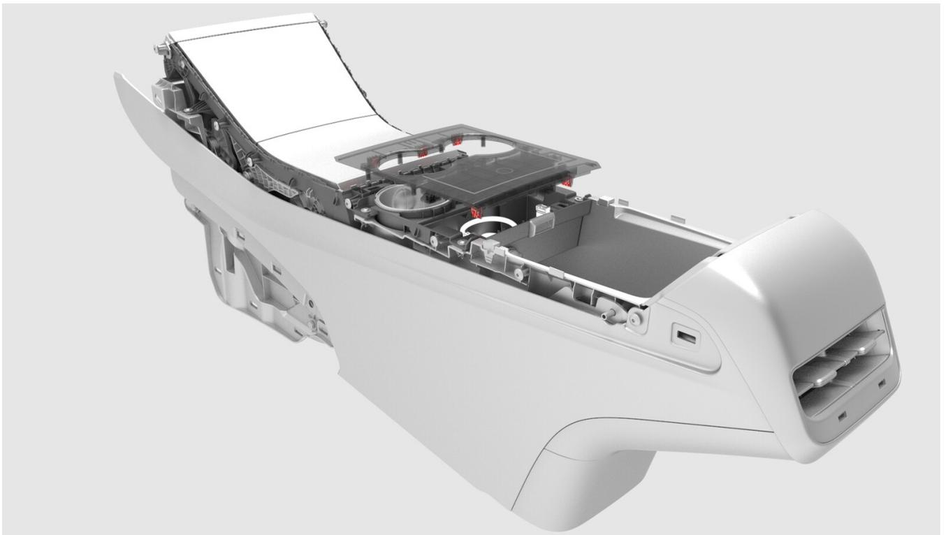
6. Disconnect the electrical harness from the security body controller module connector, and then remove the trim from the vehicle.
