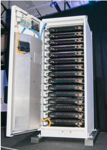
Figure 5 The Tesla PowerPack, open, with trays and cooling visible (Wood 2015)
