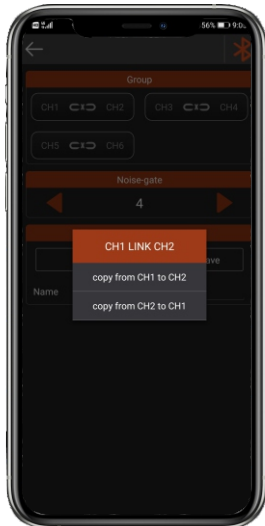
Link: Press the "system" button you can set the link channel function CH1&CH2 CH3&CH4, CH5&CH6,
