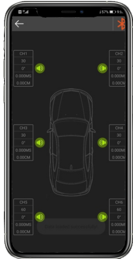
Chanel: Press Channels ico You will see the interface,you can set each channel's Gain/Phase/Time delay/Open/close volume.
