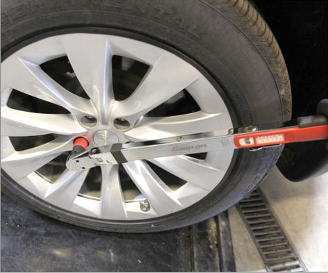
17. Fully tighten the LH rear drive unit halfshaft nut (torque 245 Nm).
