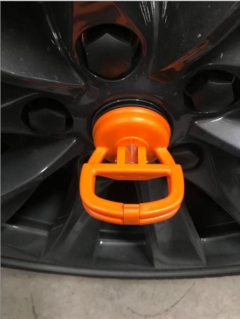
2. Use the wheel nut cover removal tool to remove the LH rear wheel lug nut covers.
