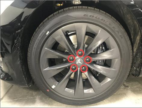
3. Loosen the LH rear wheel lug nuts.
