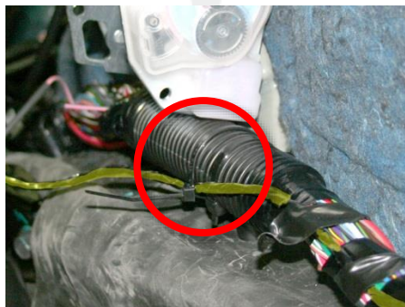
Figure 24 (TPMS harness highlighted)
