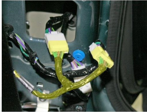
Figure 12 (TPMS harness highlighted)
