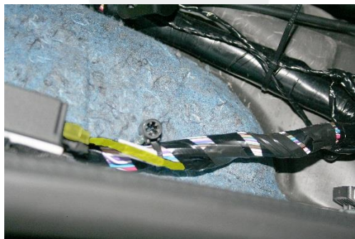
Figure 26 (TPMS harness highlighted)
