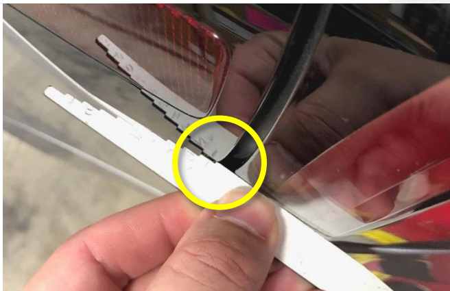
✓ Figure 2 – Overflush 1.5 mm or less
