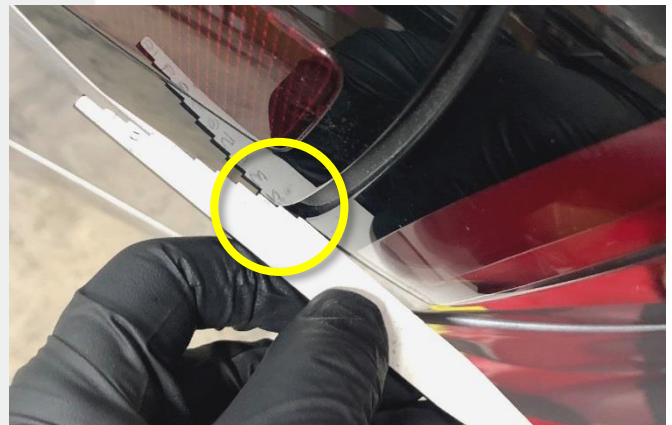
✗ Figure 3 – Overflush greater than 1.5 mm
