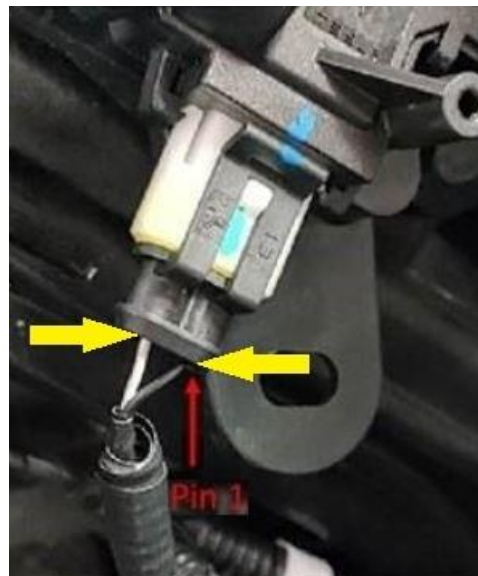
✗ Figure 3 – Incorrect wire position
