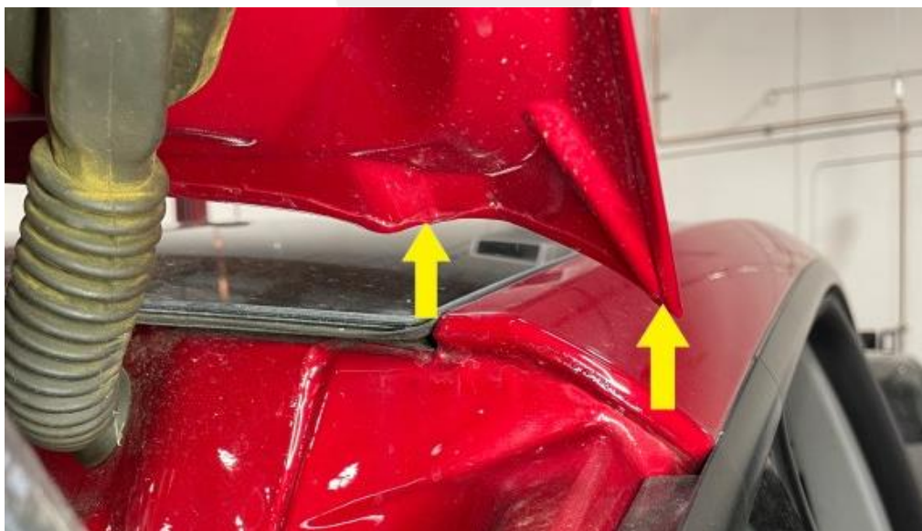
Figure 23 – Example of liftgate assembly seam
