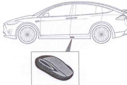
To drive Model X, place the key against the center console, immediately below the 12V power outlet, then press and hold the brake pedal to turn Model X on.
