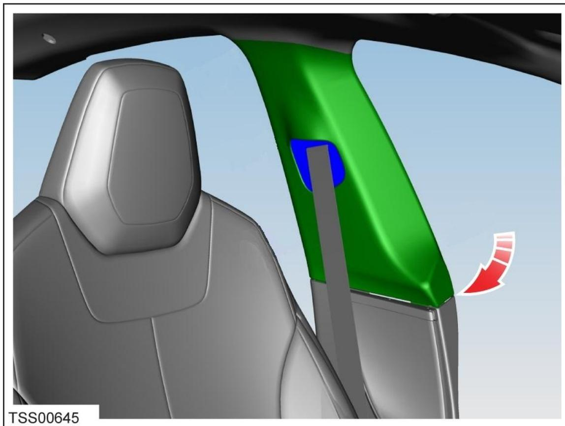
3. Allow the B-pillar upper trim to rest on the seatbelt buckle.
