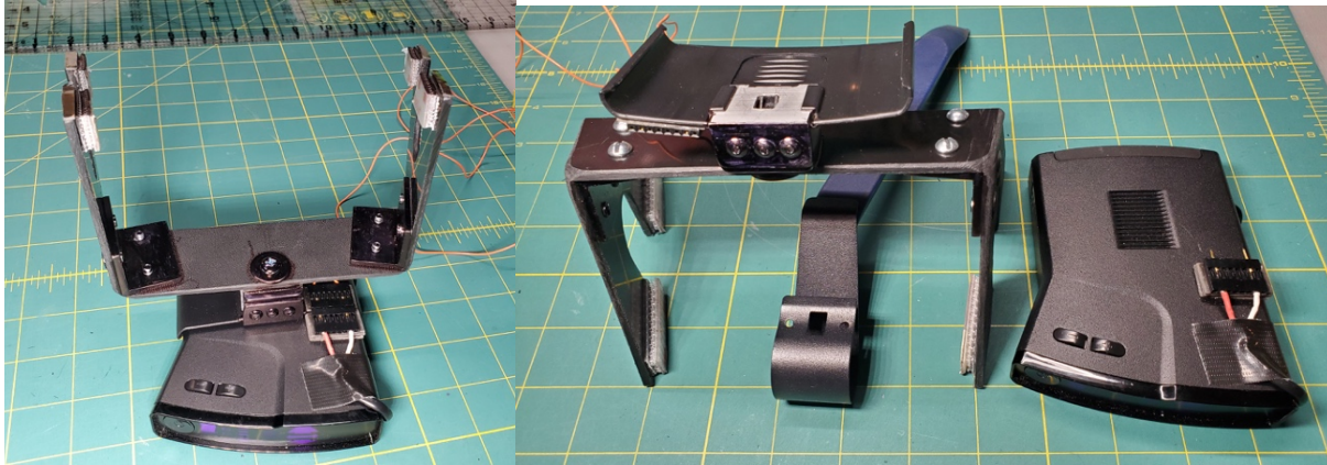
Figure 8. Quick Mount Ready to Install. At center is the unused steel clip and a blue plastic trim tool.
