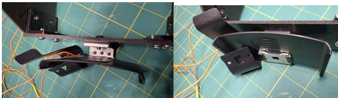
Figure 6. Attaching the Valentine Visor Mount, with Steel Spring Clip removed, to the Cross Bar via an Aluminum C-shaped part.
