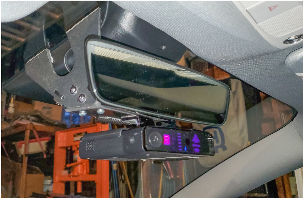
Figure 3. Completed Quick Mount Prototype. V1G2 in 2020 Tesla Model 3.
