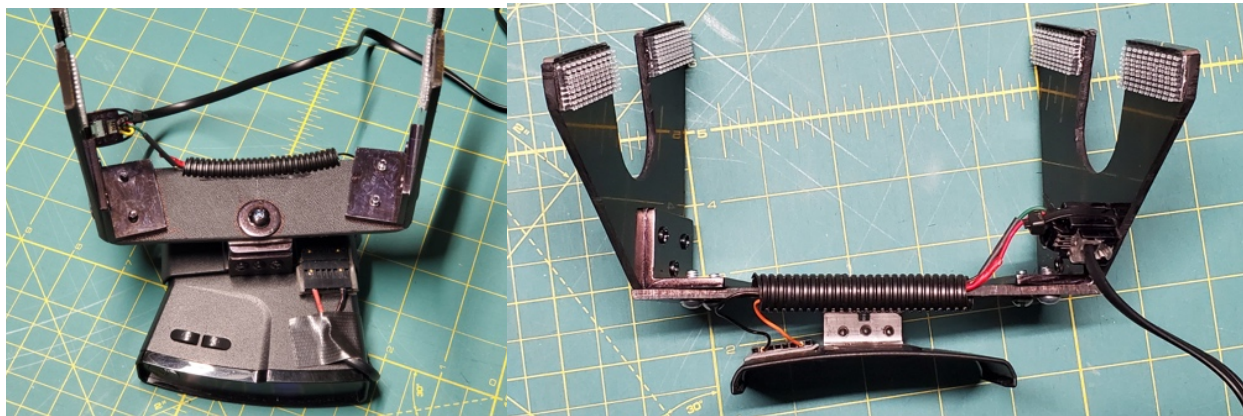
Figure 12. Quick Mount with RJ-11 Connector Attached to Left Upright. V1 power cable plugged-in
