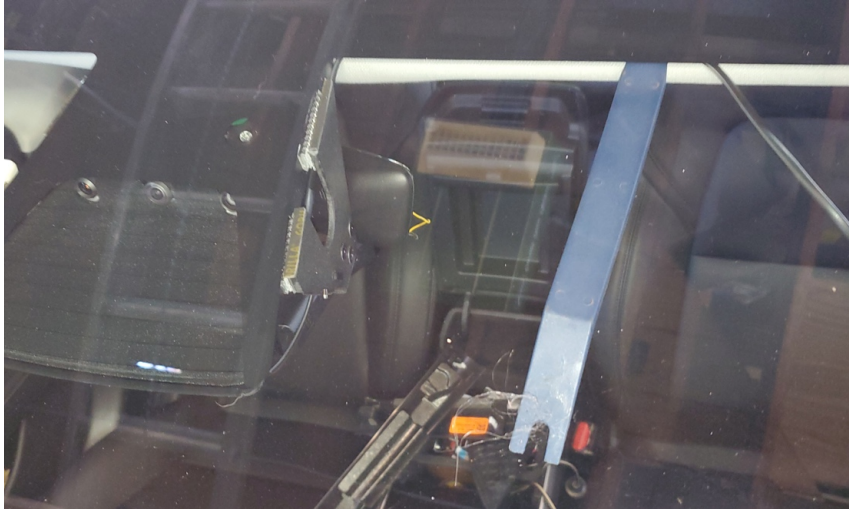
Figure 13. Tucking the Power Cable Behind the Headliner.
