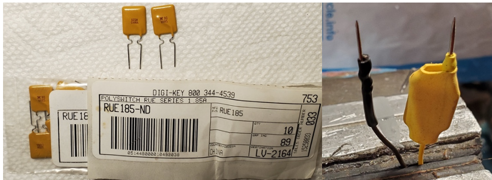
Figure 10. Polyswitch Resettable Fuse
