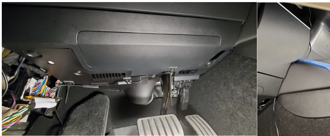
Figure 16. USB Cable Routing from Topfit Phone Mount to 12V Source
