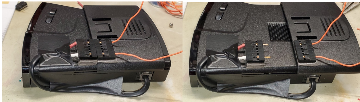
Figure 5. Quick Mount Connector on V1G2 Connected/Disconnected. Black electrical tape was later replaced with Black Gorilla Duct Tape, which sticks much better and looks like carbon fiber.
