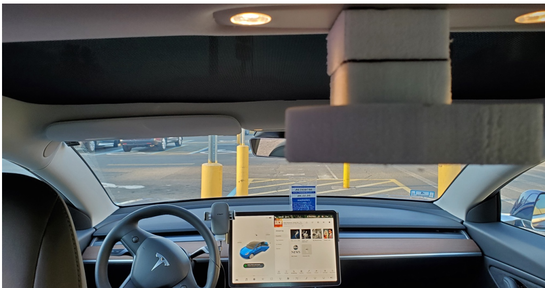
Figure 2. Rear Dome Light Location Mockup. On a flat, level parking lot from back seat.
