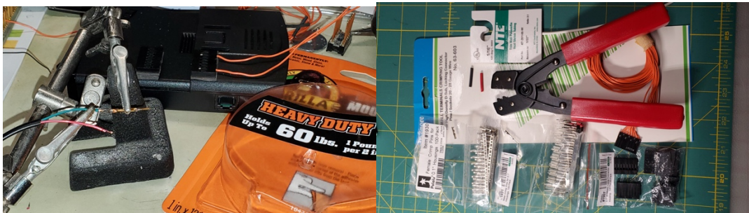
Figure 4. Using Gorilla HD Double Sided Tape to Mount the Connector Blocks, Parts & Crimp Tool Used Later.
