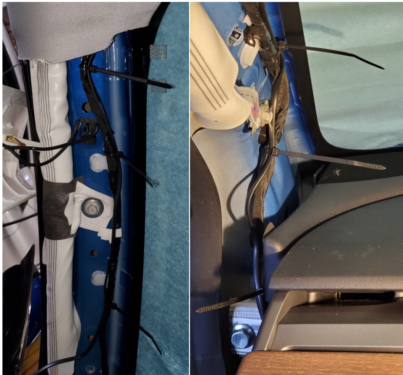
Figure 14. Attaching the Power Cable to the Existing A-Pillar Harness.
