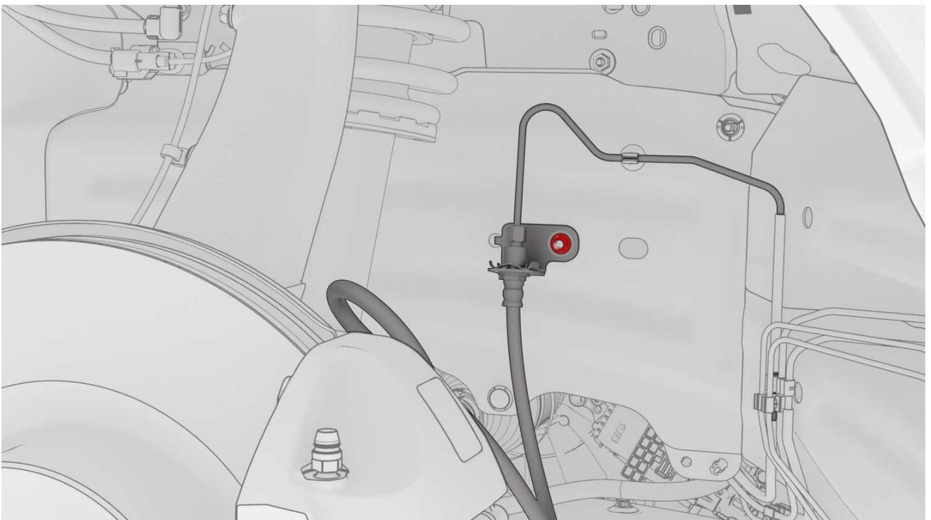
8. Remove the bolt and nyloc nut (discard the nut) that attach the front upper control arm to the knuckle.
