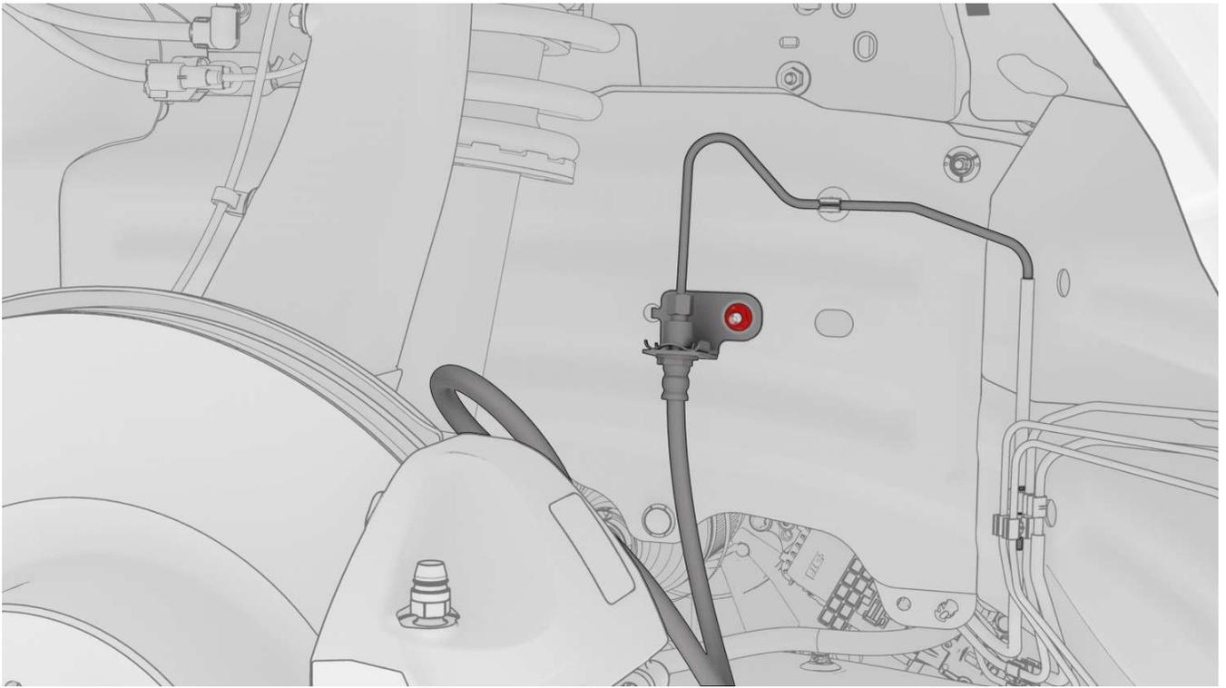
10. Install the clips (x2) that attach the front wheel speed sensor harness to the knuckle.
