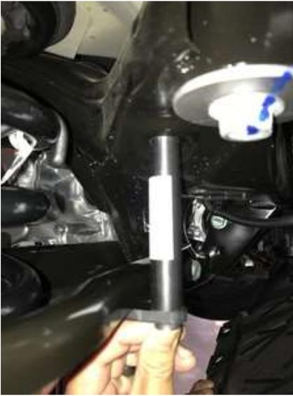
9. Measure the distance between the bottom of the quarter panel to the center of the rear axle to make sure that the rear suspension is set to ride height: The distance should measure 427 mm.
