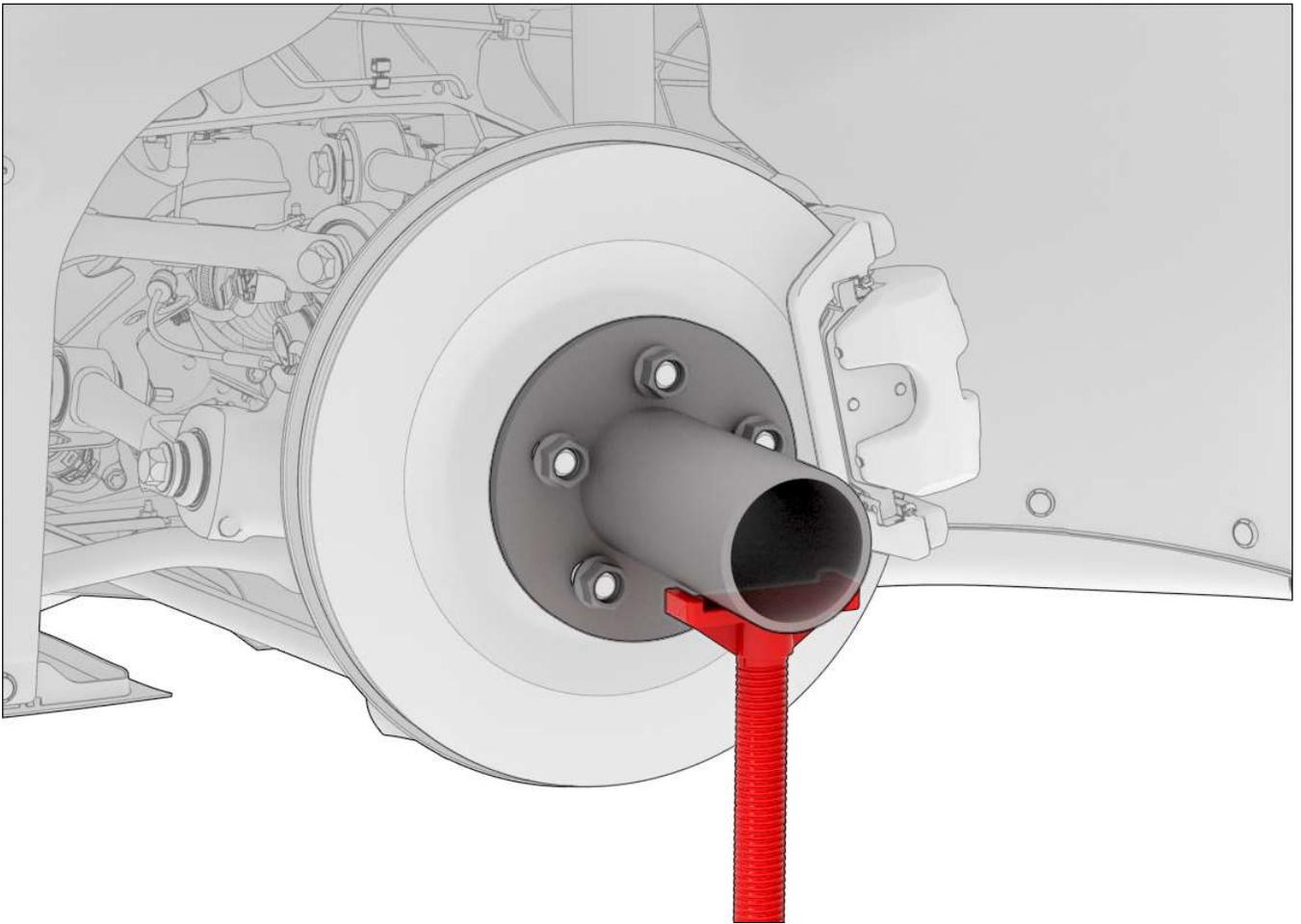
8. Locate the rear ride height torque tool insertion point in the subframe, and then insert the rear ride height torque gauge to verify that the rear suspension is set to ride height specifications. Adjust the support stand or spring compressor tool, if necessary.
